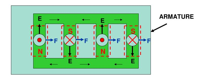
Front side stator magnets removed for clarity
