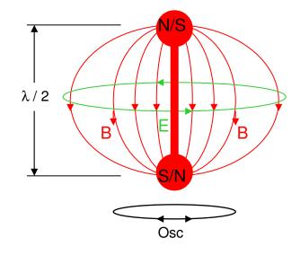
The A<sub>0</sub> magnetic potential field is in the circular (theta) direction.
