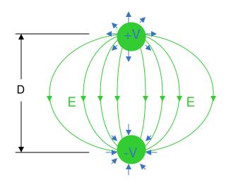
The V electric potential fields radiate outward (radial) from each pole decreasing with distance (radius). Polarity of +V field being the equal and opposite of -V field.
