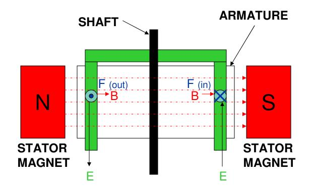
Figure legend: green= E-field, red= B-field, blue= F-field "dot"= out of page and "X"= into page
