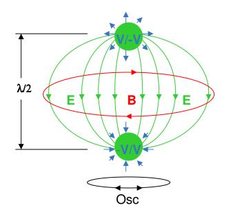
The V electric potential fields radiate outward (radial) from each pole decreasing with distance (radius). Polarity of +V field being the equal and opposite of -V field.
