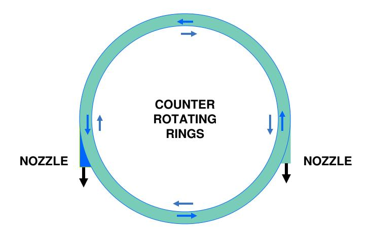
Matter is spun in counter rotating rings close to the speed of light, then the beams exit through rocket nozzles.
