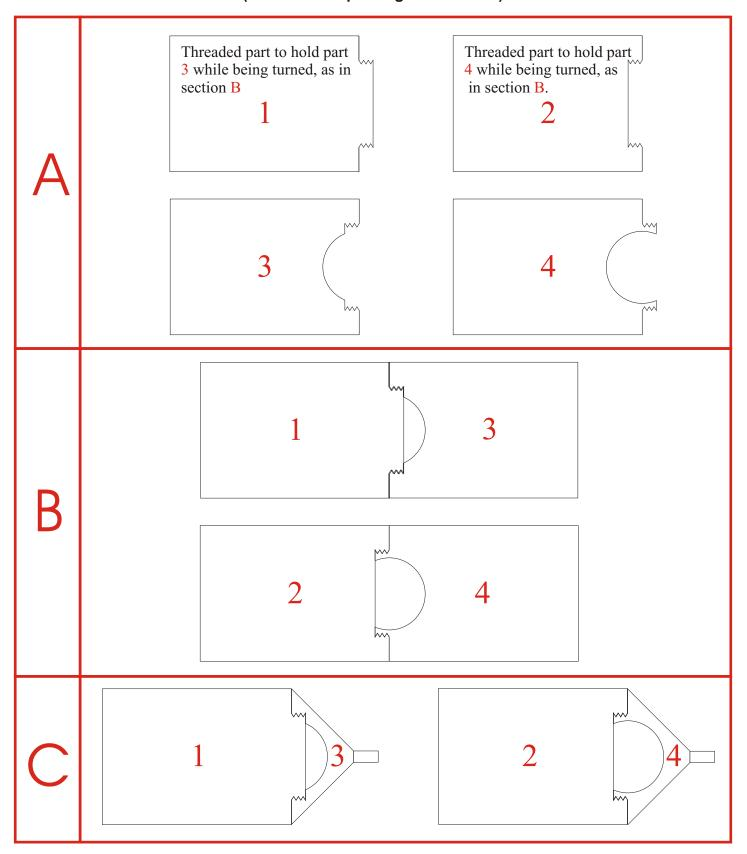
It may be necessary to begin the machining with the parts marked 1, 2, 3, 4 above in section A. With the corresponding threads machined on each end to hold the cones 3 & 4 respectively, as they are being machined.
